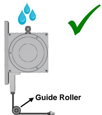
**4. The wire should not be pulled in angular. If needed, please use guide rollers.**
